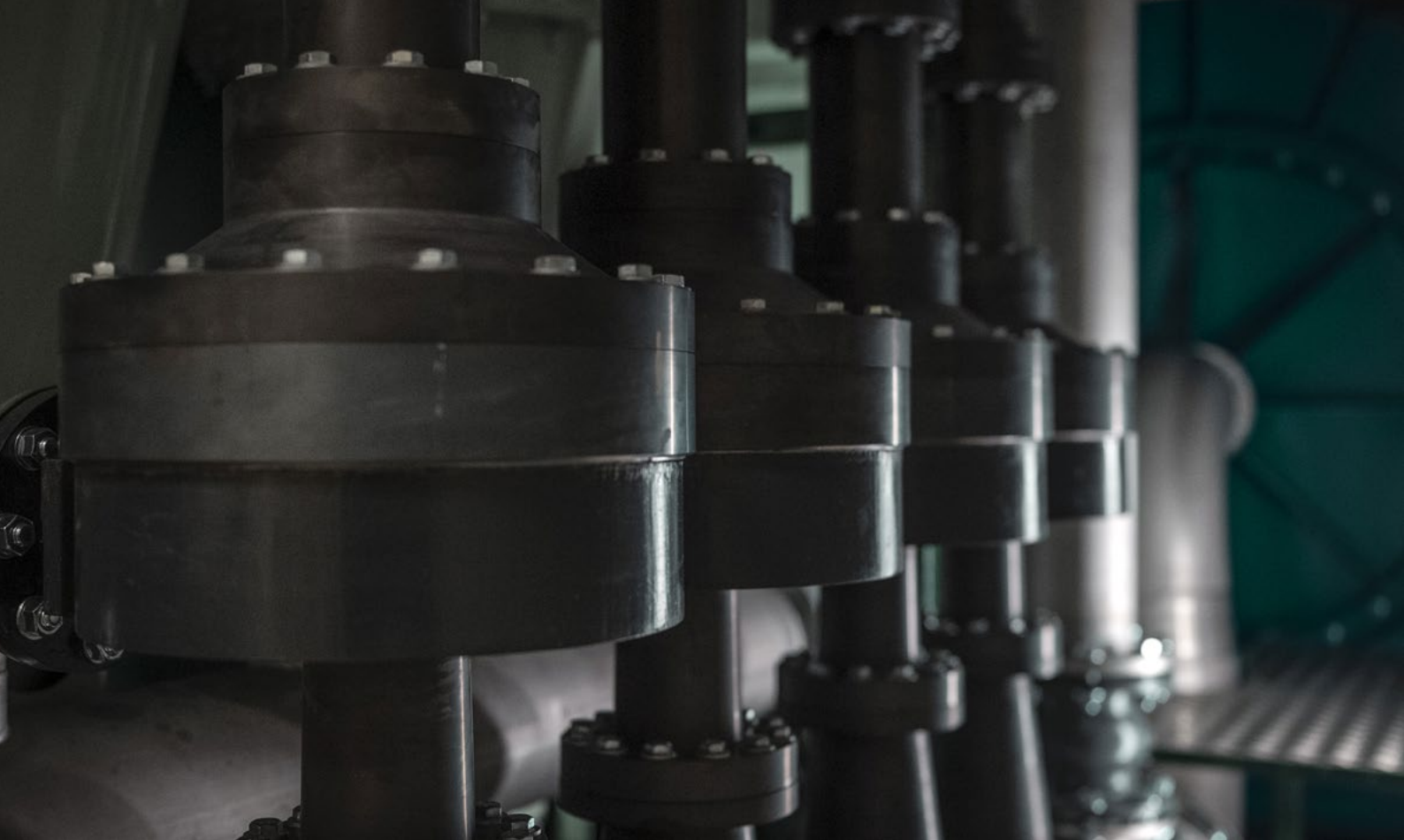
▲ Separation cores of a quad-core DC402 model.
